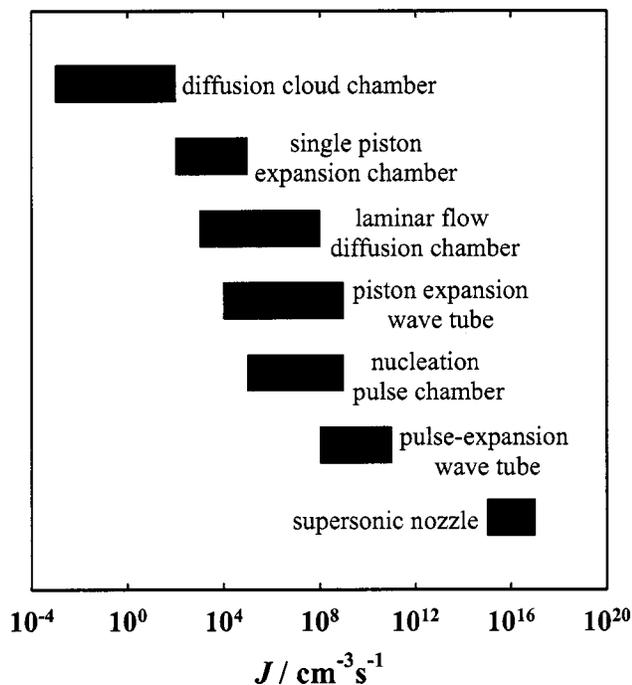
FIG. 1. Different techniques for homogeneous nucleation experiments and their respective ranges in nucleation rates  $J$ .
