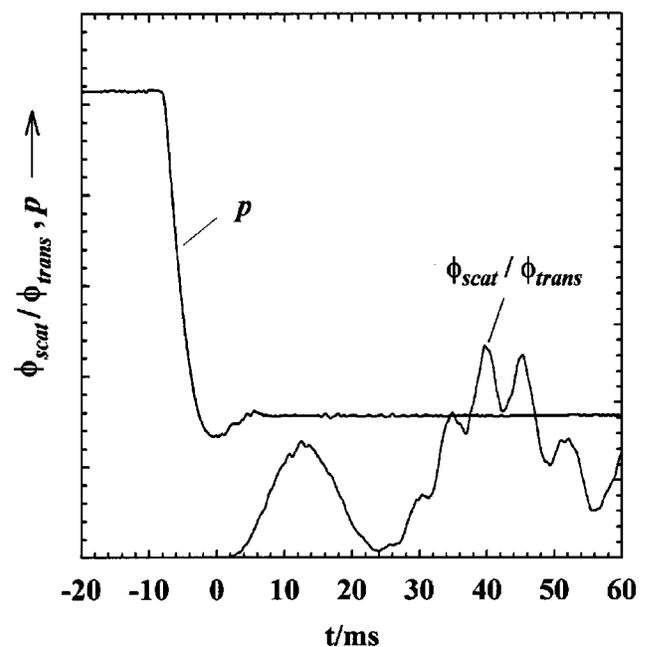
FIG. 2. Typical nucleation pulse and corresponding light scattering signal for a 1-pentanol experiment.
